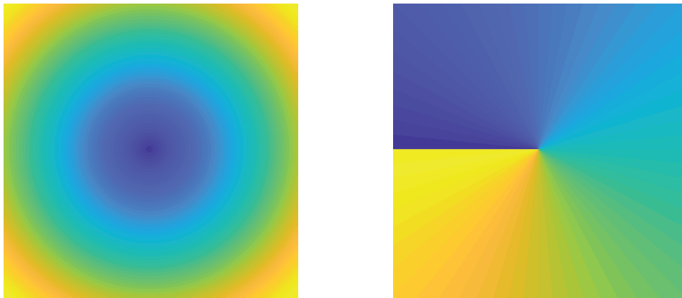
Figure 4: Representation of the complex plane z = x + iy = re^{i\theta} in Matlab. Left panel: magnitude r = |z| . Right panel: angle \theta = \arg(z)
